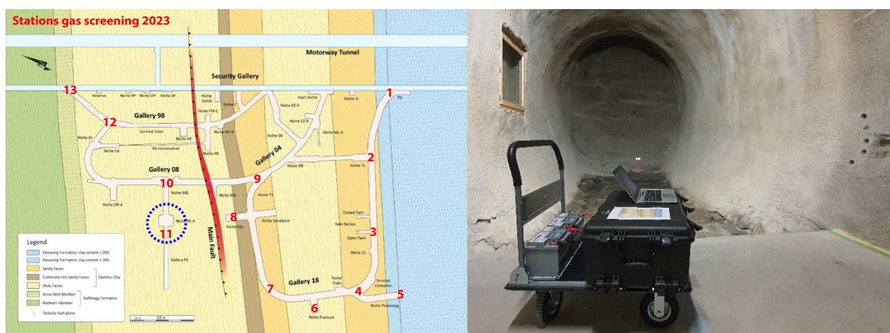
Fig. 1. Left panel: Position of the different stations where the gas screening was conducted on Nov. 16 th 2023 (picture adapted from the Mont Terri Project website: www.mont-terri.ch ). The dotted circle marks the position of the niche of the FE experiment. Right panel: miniRUEDI running on batteries in the niche Passwang (Station 5, picture by Y. Tomonaga).
