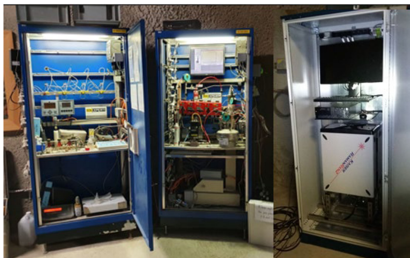
Fig. 1. Photograph of the experimental equipment of HT experiment inside the Mont Terri URL. From left to right: the water sampling module, the gas circulation module and the Raman spectrometer (photograph by M. Lundy).
